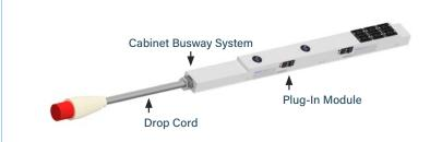
Cabinet Busway is a pre-assembled system ideal for server cabinets and industrial workbench applications. Utilizing the Plug-In Raceway components create an excellent configuration for applications that require higher power density, multiple types of receptacles and future flexibility.
