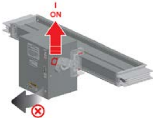
Front door is opened, the Main Device can't On status
